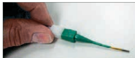
Plastic tool with contact in proper position.
