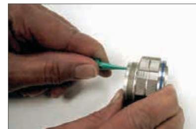
Plastic tool with contact in proper position.
